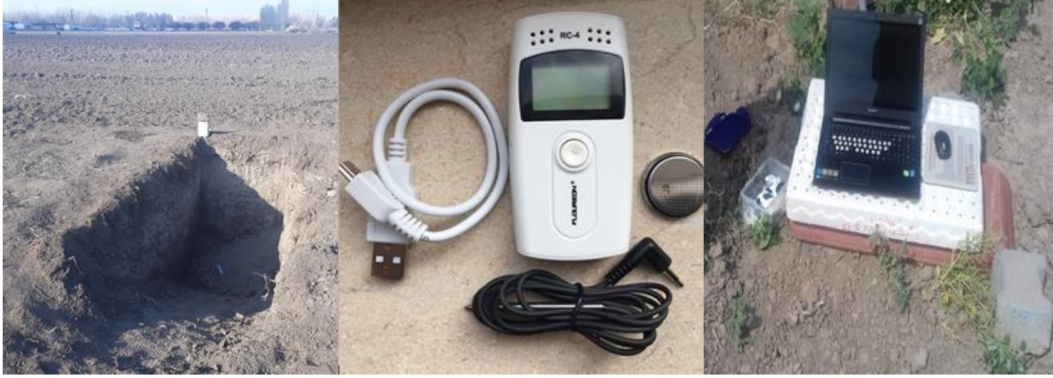
FIGURE 2. Placing the thermal sensors (Elitech RC-4 Mini temperature data logger) in soil profile
